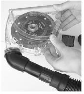
Adjust the depth of the 6. CutBuddie as needed by pushing down on the tab located on the side.
