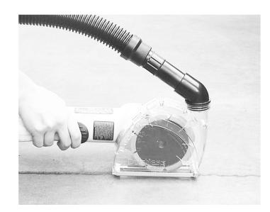
Follow Installation steps and install crack • chasing wheel.
